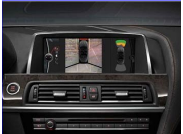
Illustration 5: Merged Image: Top, Rear , and Side View Camera
