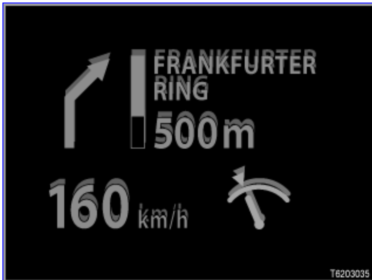
Illustration 14: HUD Image projected on a conventional windscreen
